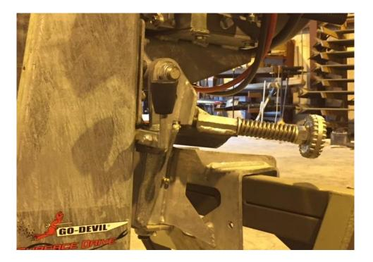
EZ Trim Lever should be placed in the down position shown below when you need to lower your trim height because of extremely low water situations (this will give you 5" of drop in prop height) and returned to the upright position once you have returned to deeper water.
