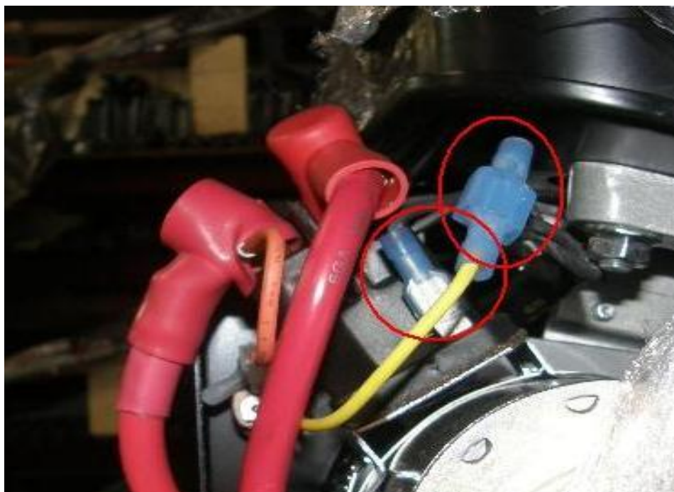
Briggs & Stratton 6.5hp Mercury Switch Wire Connections
