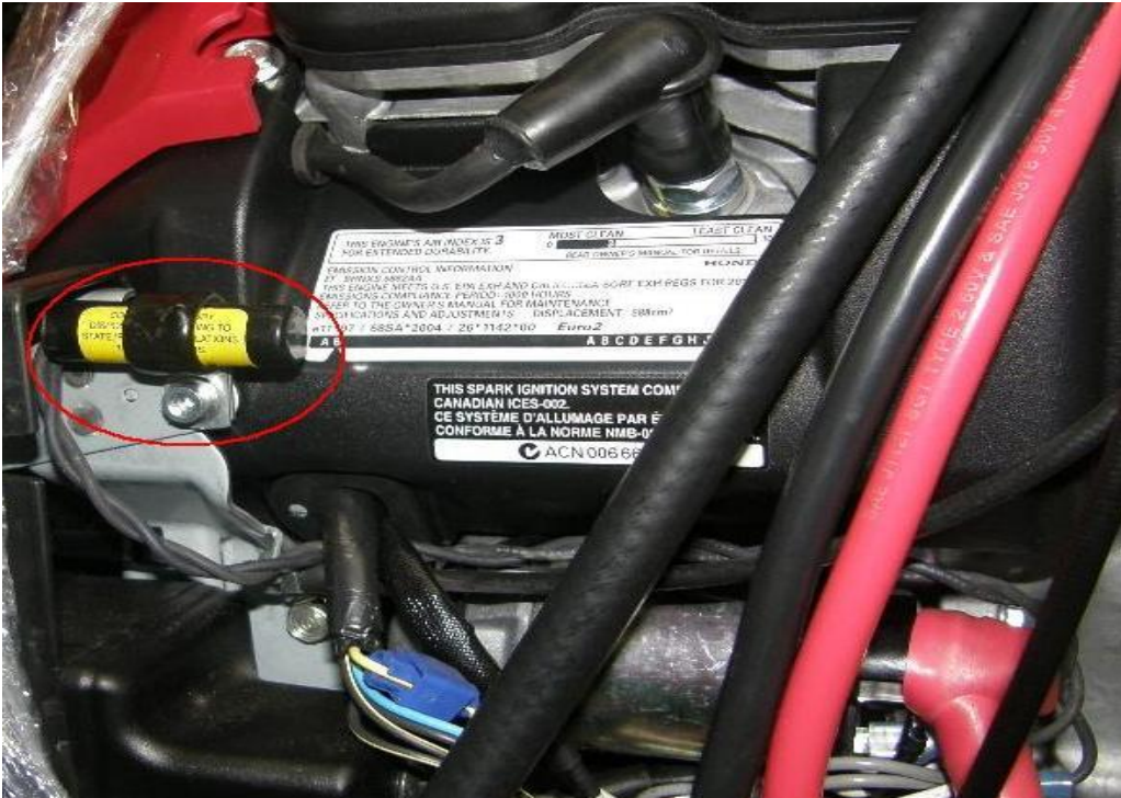
Honda GX630/690 (20, 22hp) Mercury Switch Mount Location
