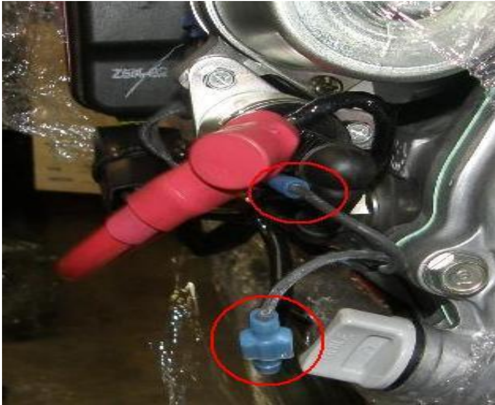
Honda 9hp Mercury Switch Wire Connection
