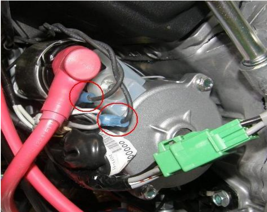
Honda GX630/690 (20, 22hp) Mercury Switch Wire Connection
