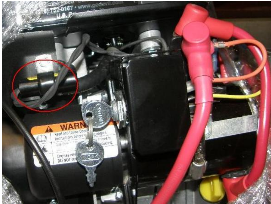
Briggs & Stratton 6.5hp Mercury Switch Mount Location
