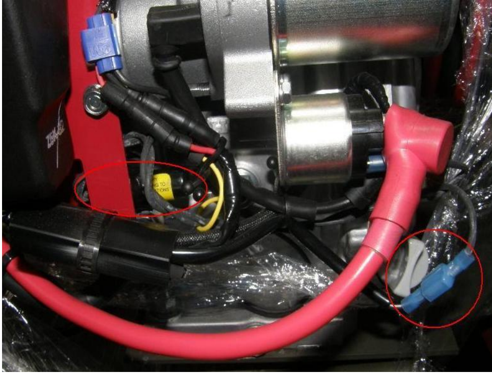
Honda 9hp Mercury Switch Mount Location
